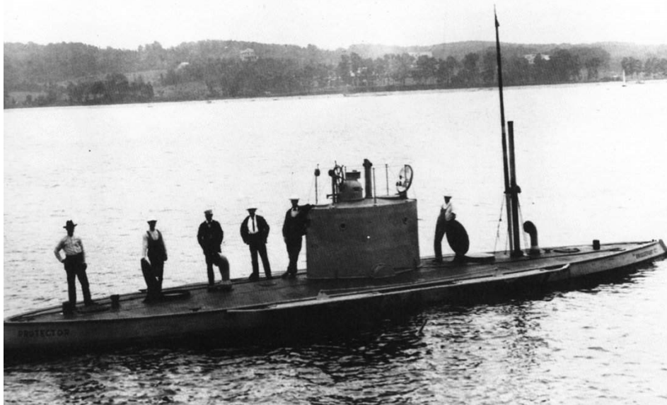
Lake's Protector was his rival to the Electric Boat's Fulton (A prototype of the Adder class (SS-2-8) submarines). She is clearly designed as a submersible surface ship, with high freeboard, a wide flat deck, and a large conning tower. The pipe aft is a exhaust engine. Lake sold this type of submarine to Russia.
